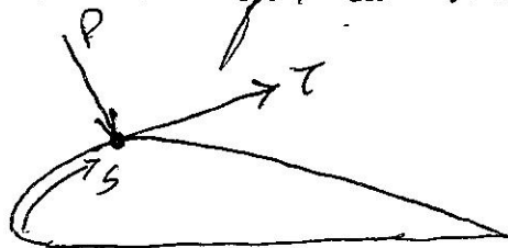
Fig: Illustration of Pressure & shear stresses on an aerodynamic surface.
